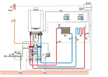
EMC-M... MI with 1 underfloor circuit and 1 direct circuit. DWH produced by a solar calorifier with mixing valve kit (package HR 84)
