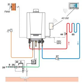
EMC-M 24/BS 80 with 1 direct circuit + DHW production circuit, controlled by a programmable room thermostat (wire)
