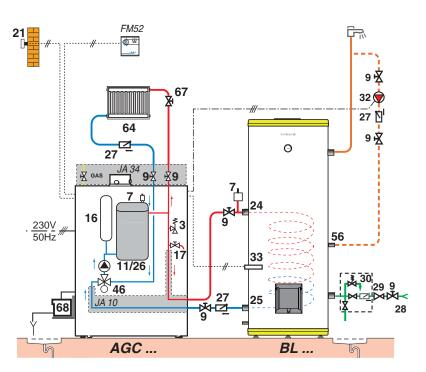
AGC.../V 100 HL with 1 underfloor heating circuit (direct), outside sensor, interactive remote control (wire)
