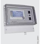
VM iSystem wall-hung control unit - Package AD 281 The VM iSystem electronic control system, incorporated in a wall-mounted box, is used to manage and control two heating circuits and a DHW circuit and each of the heating circuits may be a direct circuit or a circuit with motorised 3-way mixing valve.
