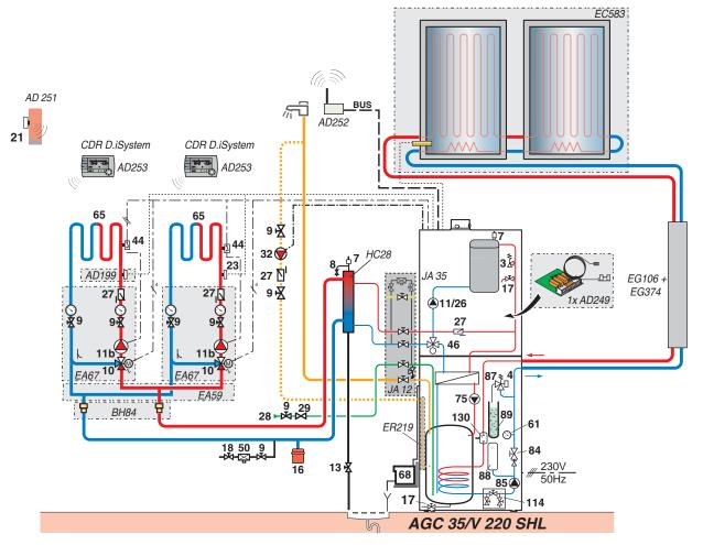
Note: in this example, the limited manometric height of the pump fitted to the AGC 35 requires the use of a disconnecting cylinder (option HC 28).
